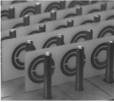
(a) Photograph of the composite thin wire arrays and SRRs that exhibits a negative refractive index (Smith et al. 2000). (Courtesy of D. R. Smith.)
