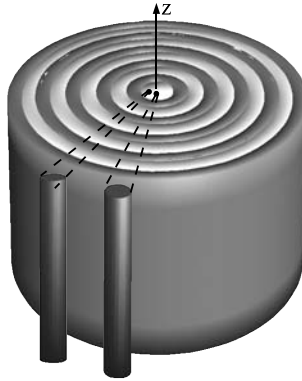
Figure 9.11 A cylindrically layered medium with alternate cylindrical layers of a negative dielectric medium (gray) and a positive medium (white) acts as an indefinite effective medium. This can be utilized to project out the near-field information of two small sources embedded within the innermost layer to the space outside the layered cylindrical system. The image so produced has a magnification and may be outcoupled to the far-field propagating modes easily.
